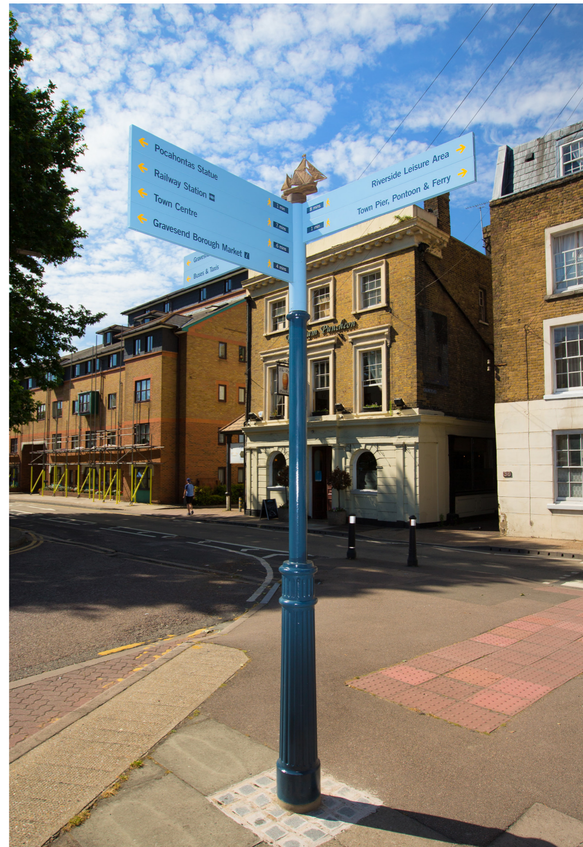
Example of Octopus post adapter, used to connect directional fingers and telescopic spline to existing cast sign post.
