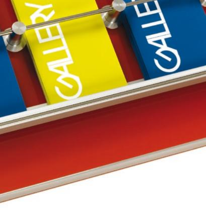
Holders can be made to fit any combination of brochures, typical brochure formats include; A4, 1/2A4, 1/3A4, A5, A6 etc. Brochure holders are formed from turned aluminium bosses, with a horizontal rod to keep the brochures upright and an extruded aluminium tray. Brochure holders come in silver as standard. The tray has a capacity of 25mm.
